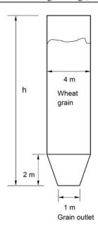
A circular grain silo with conical bottom, as shown in figure, is filled with wheat (true density 1200 kg m<sup>-3</sup>) with porosity of 0.6. Five hundred metric tonne of wheat fills 80% of its capacity (by volume). The total height (h) of the silo from its grain outlet end in m is \_\_\_\_\_\_\_.
