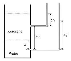
The distance (x in cm, rounded off to the first decimal place) of the interface from the point at which the lower L-tube is connected is
