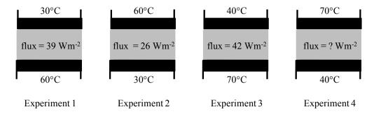
What is the steady state heat flux (in W  $m^{-2}$ ) with the top plate at  $70^{\circ}$ C and the bottom plate at  $40^{\circ}$ C?
