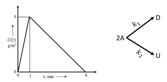
The rate constants are  $k_1 = 0.2$  Liter/(mol min) and  $k_2 = 0.3$  Liter/(mol min). Pure A is fed to the reactor at a concentration of 2 mol/Liter. Using the segregated model, the percentage conversion in the reactor is \_\_\_\_\_\_ (rounded off to the nearest integer).
