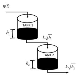
At steady state operation, the water inlet flow rate is  $q_{ss} = 16$  cm<sup>3</sup>/s. The transfer function relating the deviation variables  $\,\tilde{h}_{\!\!2}\,$  (cm) to flow rate  $\,\tilde{q}\,$  (cm³/s) is,
