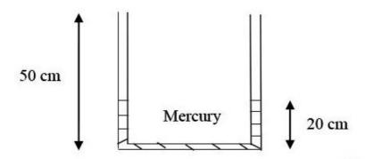
If 5 cm<sup>3</sup> of water is added to the right limb, the new height (in cm, up to two decimal places) of mercury in the LEFT limb will be
