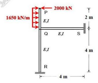
The rotation (in degrees, up to one decimal place) at the rigid joint Q would be \_\_\_\_\_
