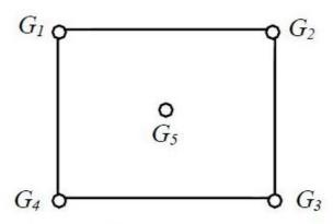
During a month, the precipitation at these gauges is measured as  $G_1 = 300$  mm,  $G_2 = 285$  mm,  $G_3 = 272$  mm,  $G_4 = 290$  mm and  $G_5 = 288$  mm. The average precipitation (in mm, up to one decimal place) over the catchment during this month by using the Thiessen polygon method is
