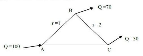
The head loss in each pipe is given by  $h_f = rQ^{1.8}$ , with the variables expressed in a consistent set of units. The value of r for the pipe AB is 1 and for the pipe BC is 2. If the discharge supplied at the point A (i.e., 100) is equally divided between the pipes AB and AC, the value of r (up to two decimal places) for the pipe AC should be
