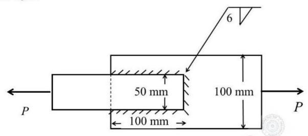
The permissible stresses in the plate and the weld are 150 MPa and 110 MPa, respectively. Assuming the length of the weld shown in the figure to be the effective length, the permissible load P (in kN) is
