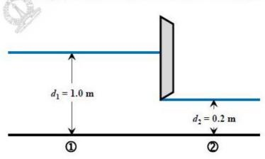
It is observed that the depth of flow is 1.0 m upstream of the gate, while the depth is 0.2 m downstream of the gate. Assuming a smooth flow transition across the sluice gate, i.e., without any energy loss, and the acceleration due to gravity as 10 m/s², the discharge (in m³/s, up to two decimal places) passing under the sluice gate is \_\_\_\_\_
