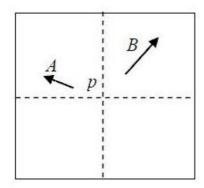
The length of the image of the tower A on the photograph is 1.5 cm and of the tower B is 2.0 cm. The distance of the top of the tower A (as shown by the arrowhead) is 4.0 cm and the distance of the top of the tower B is 6.0 cm, as measured from the principal point p of the photograph. If the height of the tower B is 80 m, the height (in meters) of the tower A is \_\_\_\_\_\_
