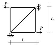
For the loads shown on the truss, the statement that correctly represents the nature of forces in the members of the truss is:
