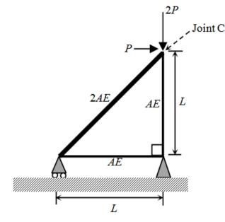
Given that  $E = 2 \times 10^{11}$  N/m<sup>2</sup>, A = 10 mm<sup>2</sup>, L = 1 m and P = 1 kN. The horizontal displacement of Joint C (in mm, up to one decimal place) is \_\_\_\_\_
