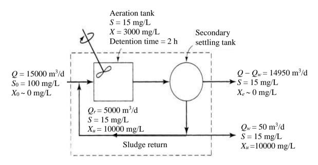
$S_0$ , S = readily biodegradable soluble BOD, mg/L Q,  $Q_r$ ,  $Q_w$  = flow rates, m<sup>3</sup>/d  $X_0$ , X,  $X_e$ ,  $X_u$  = microorganism concentrations (mixed-liquor volatile suspended solids or MLVSS), mg/L
