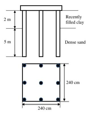
The negative frictional load (in kN, up to two decimal places) acting on the pile group is
