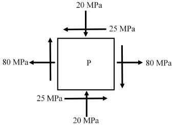
By how much angle ( $\theta$ ) in *degrees* the stress element should be rotated in order to get the planes of maximum shear stress?
