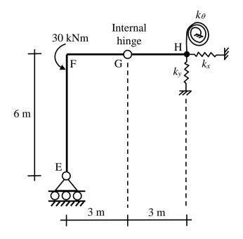
For the externally applied moment of 30 *kNm* at node F, the rotation (in *degrees*, *round off to 3 decimals*) observed in the rotational spring at node H is \_\_\_\_\_
