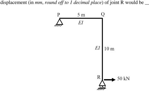
flexural rigidity, EI, of each member is  $10^6 kNm^2$ . Under the applied load, the horizontal
