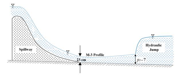
The flow enters as an M-3 profile in the long wide rectangular channel with bed slope =  $\frac{1}{1800}$  and Manning's n = 0.015. A hydraulic jump is formed at a certain distance from the foot of the spillway. Assume the acceleration due to gravity,  $g = 9.81 \text{ m/s}^2$ . Just before the hydraulic jump, the depth of flow  $y_1$  (in *m*, round off to 2 decimal places) is \_\_\_\_\_
