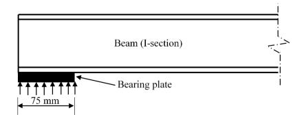
As per IS: 800-2007, the web bearing strength (in *kN*, *round off to 2 decimal places*) of the beam is \_\_\_\_\_
