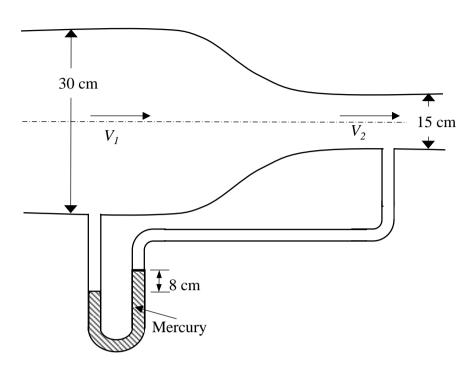
When the water flows, the differential manometer shows a deflection of 8 *cm* of mercury (*Hg*). The values of specific gravity of mercury and water are 13.6 and 1.0, respectively. Consider the acceleration due to gravity,  $g = 9.81 \text{ m/s}^2$ . Assuming frictionless flow, the flow rate (in  $m^3/s$ , round off to 3 decimal places) through the duct is \_\_\_\_\_
