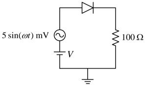
For  $\omega = 2 \times 10^6$  rad/s, the amplitude of the small-signal component of diode current (in  $\mu$ A, correct to one decimal place) is \_\_\_\_\_.
