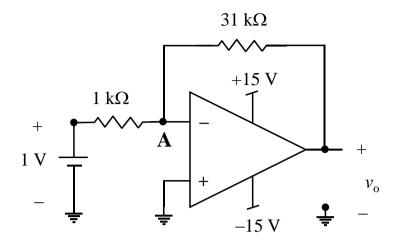
In the above circuit, assume the op-amp to be ideal. The voltage (in volts, correct to one decimal place) at node **A**, connected to the negative input of the op-amp as indicated in the figure is \_\_\_\_\_\_.
