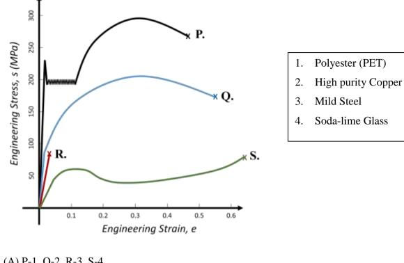
Q.31 Match the four tensile stress-strain curves (P,Q, R, S) with the materials listed in the box:
