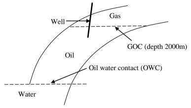
The static oil pressure gradient is 0.08 bar/m in the pay zone. If a constant hydrostatic pressure gradient of 0.1 bar/m prevails throughout the subsurface, then the thickness of the oil column is \_\_\_\_\_m (round off to 1 decimal place).
