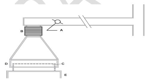
Fig: 2.4 Canopy (thimble) unit for ducting a Class II, Type A BSC (A) balancing damper; (B) flexible connector to exhaust system; (C) cabinet exhaust HEPA filter housing; (D) canopy unit; (E) BSC. Note: There is a 1" gap between the canopy unit (D) and the exhaust filter housing (C), through which room air is exhausted. (BMBL 5<sup>th</sup> edition)
