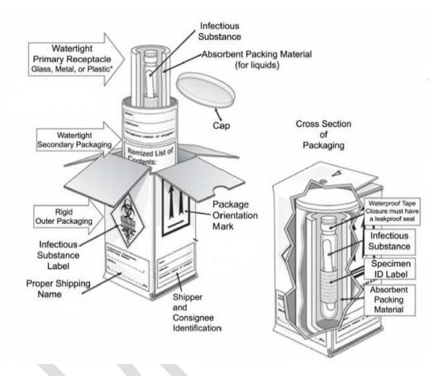
Fig 7.1. Triple packaging system
