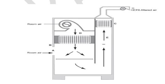
**Figure 2.6. The Class II, Type B2 BSC** (A) front opening; (B) sash; (C) exhaust HEPA filter; (D) supply HEPA filter; (E) negative pressure exhaust plenum. *Note:* The carbon filter in the exhaust system is not shown. The cabinet needs to be hard connected to the building exhaust system. (BMBL, 5<sup>th</sup> edition)
