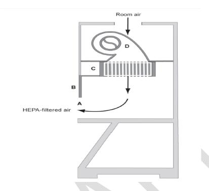
**Fig2.8.** The vertical laminar flow "clean bench" (A) front opening; (B) sash; (C) supply HEPA filter; (D) blower. *Note:* Some vertical flow clean benches have recirculated air through front and/or rear perforated grilles. (BMBL 5<sup>th</sup> edition)
