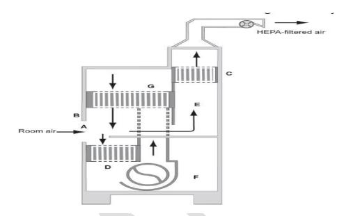
**Fig 2.5 The Class II, Type B1 BSC (classic design)** (A) front opening; (B) sash; (C) exhaust HEPA filter; (D) supply HEPA filter; (E) negative pressure dedicated exhaust plenum; (F) blower; (G) additional HEPA filter for supply air. Note: The cabinet exhaust needs to be hard connected to the building exhaust system. (BMBL 5<sup>th</sup> edition)
