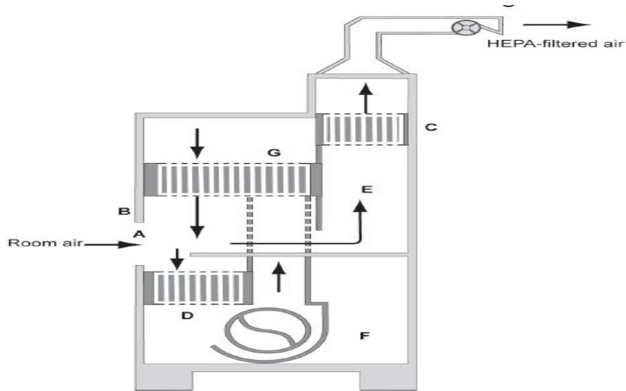
**Fig 2.5 The Class II, Type B1 BSC (classic design)** (A) front opening; (B) sash; (C) exhaust HEPA filter; (D) supply HEPA filter; (E) negative pressure dedicated exhaust plenum; (F) blower; (G) additional HEPA filter for supply air. Note: The cabinet exhaust needs to be hard connected to the building exhaust system. (BMBL 5<sup>th</sup> edition)
