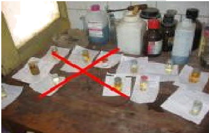
**Fig 3.3: Do not keep specimens on request forms**
