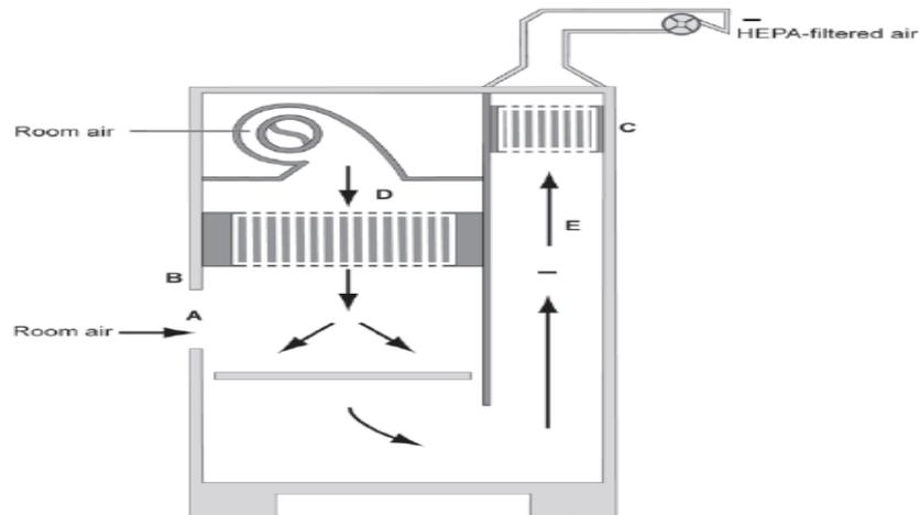
**Figure 2.6. The Class II, Type B2 BSC** (A) front opening; (B) sash; (C) exhaust HEPA filter; (D) supply HEPA filter; (E) negative pressure exhaust plenum. Note: The carbon filter in the exhaust system is not shown. The cabinet needs to be hard connected to the building exhaust system. (BMBL, 5<sup>th</sup> edition)
