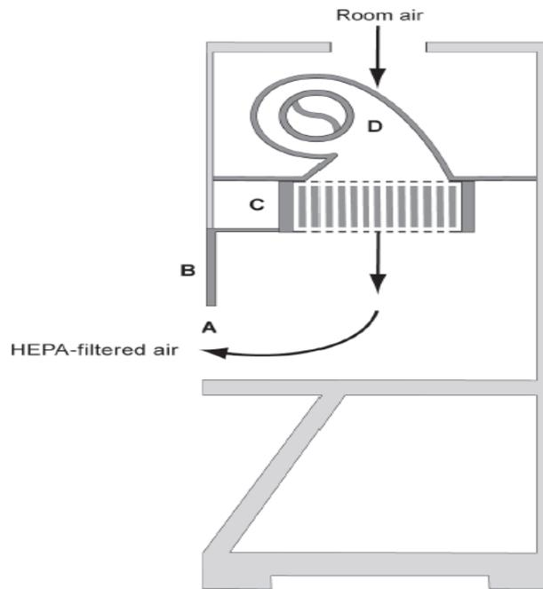
**Fig2.8. The vertical laminar flow “clean bench”** (A) front opening; (B) sash; (C) supply HEPA filter; (D) blower. *Note:* Some vertical flow clean benches have recirculated air through front and/or rear perforated grilles. (BMBL 5<sup>th</sup> edition)
