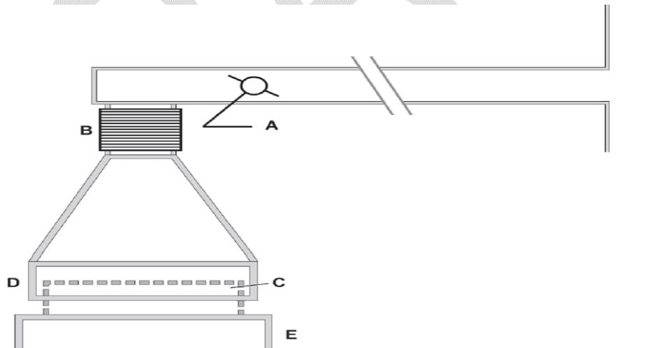
**Fig: 2.4 Canopy (thimble) unit for ducting a Class II, Type A BSC (A) balancing damper; (B) flexible connector to exhaust system; (C) cabinet exhaust HEPA filter housing; (D) canopy unit; (E) BSC. Note: There is a 1" gap between the canopy unit (D) and the exhaust filter housing (C), through which room air is exhausted. (BMBL 5<sup>th</sup> edition)**
