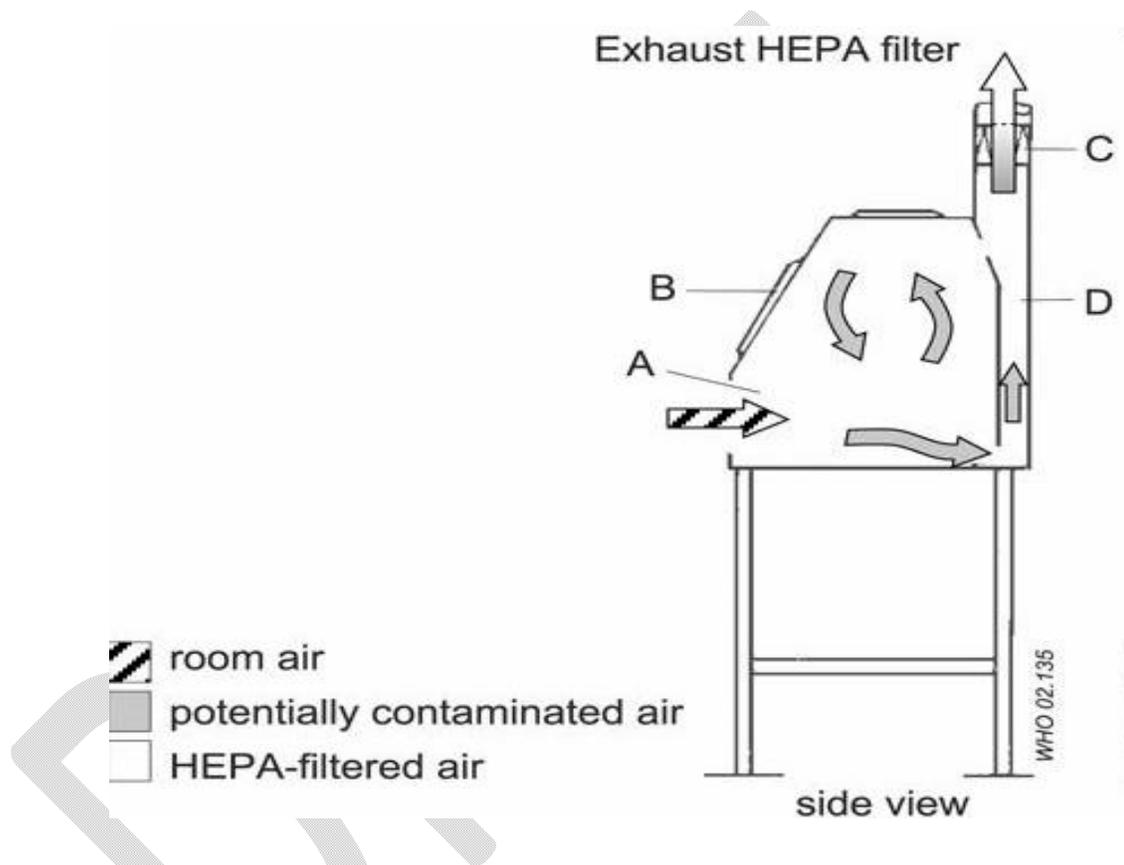
**Fig: 2.1 Schematic representation of a Class I biological safety cabinet.** A: front opening, B: sash, C: exhaust HEPA filter, D: exhaust plenum. (BMBL 5<sup>th</sup> edition)
