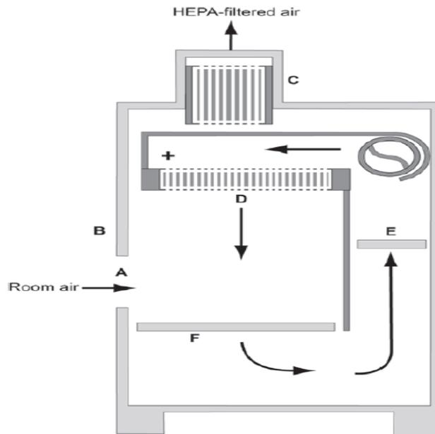
**Fig: 2.3 The table top model of a Class II, Type A2 BSC (A) front opening; (B) sash; (C) exhaust HEPA filter; (D) supply HEPA filter; (E) positive pressure common plenum; (F) negative pressure plenum. Note: The A2 BSC should be canopy connected to the exhaust system. (BMBL 5<sup>th</sup> edition)**
