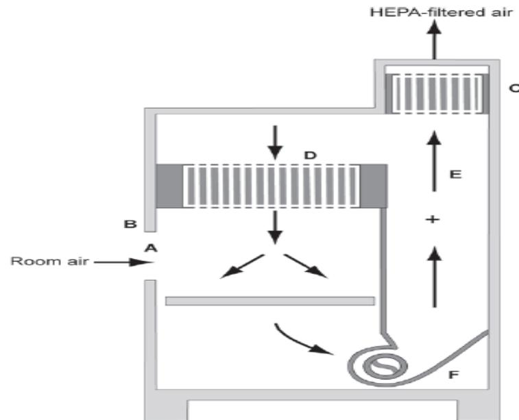
**Fig: 2.2 Schematic representation of a Class II A1 biological safety cabinet.** A: front opening, B: sash, C: exhaust HEPA filter, D: supply HEPA filter, E: common plenum, F: blower (BMBL 5<sup>th</sup> edition)
