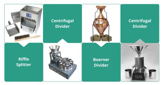
*Figure-15 : Devices used to divide and prepare a representative laboratory sample from the bulk sample.*
