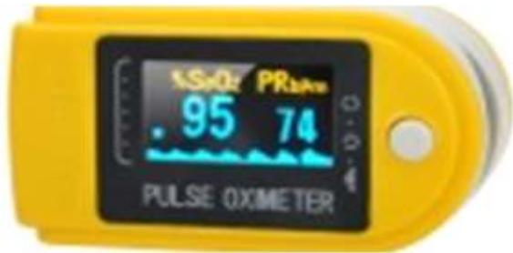
Figure.11 : Pulse Oximeter. (a) Pulse oximetry shows oxygen saturation, heart rate
